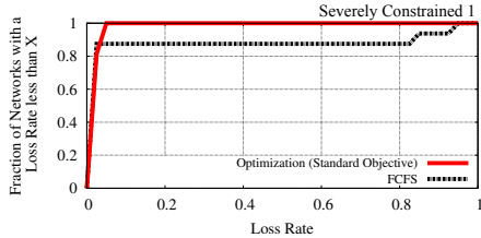
Fig. 32. Our optimization avoid significantly higher loss rates that are observed in FCFS.
