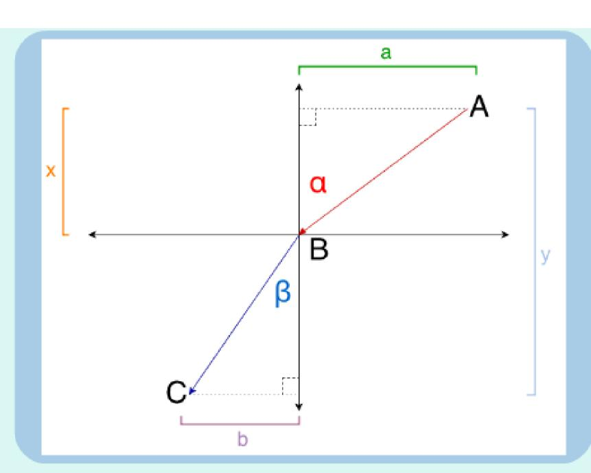
Distance = AB+BC =  $\sqrt{(a^2+x^2)} + \sqrt{(b^2+(y-x)^2)}$ Velocity = distance/time
