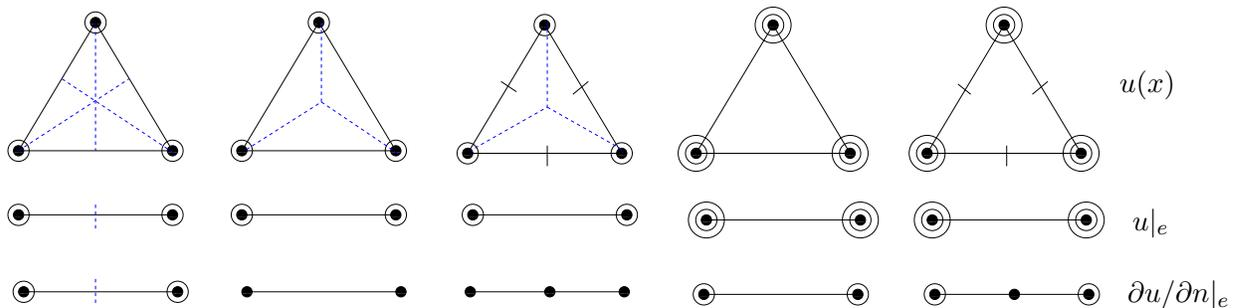
FIG. 1.1. Composite  $\mathcal{P}_2$ , reduced HCT, HCT, Bell, and Argyris,  $C^1$  triangles
