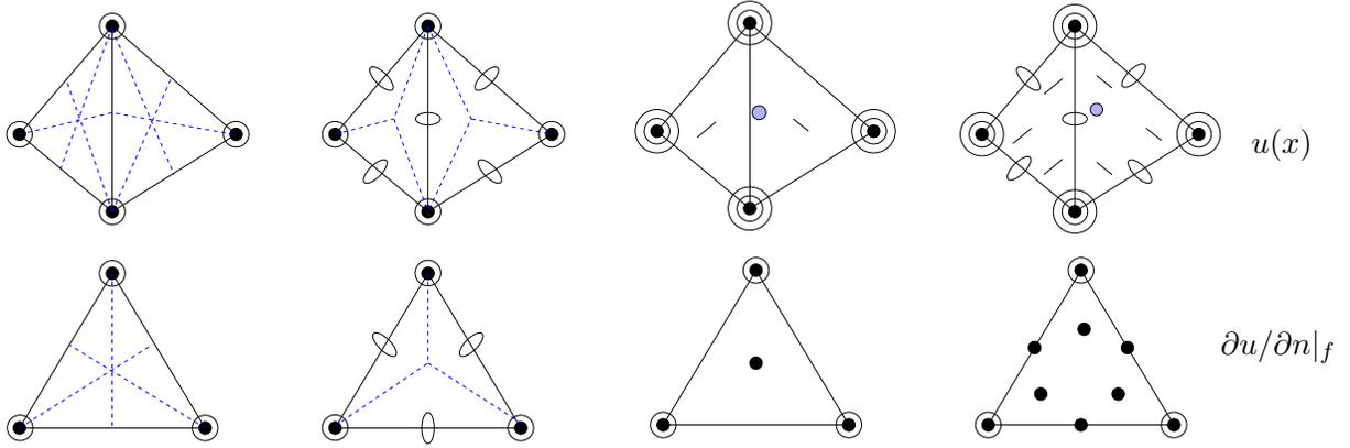
FIG. 1.2. Composite  $\mathcal{P}_2$ ,  $\mathcal{P}_3$ , reduced  $\mathcal{P}_5$ , and  $\mathcal{P}_5$ ,  $C^1$  tetrahedra.
