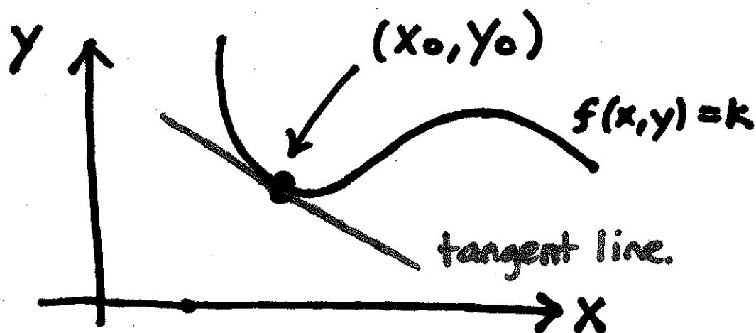
Equation of Contour :  $F(x, y) = f(x, y) - k = 0.$
