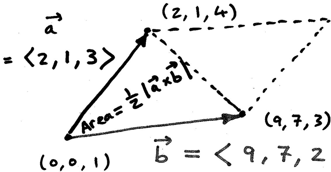
$$\vec{a} \times \vec{b} = \begin{array}{ccccccc} & i & j & k & i & j & \\ & / & \backslash & / & \backslash & / & \backslash \\ 2 & & 1 & 3 & & 2 & 1 \\ 9 & & 7 & 2 & & 9 & 7 \end{array}$$
