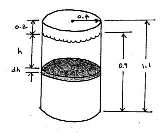
The diagram shows the physical situation. We will start by calculating the work that must be done to lift the shaded slice of hot chocolate to the top of the urn, and then use an integral to calculate the total work.
