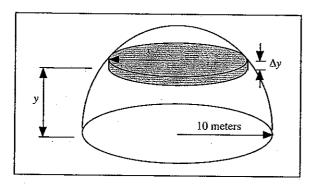
Consider the shape shown in the diagram. This shape is the top half of a sphere with a radius of 10 meters. If you look at the shape "side on" then it looks like the top half of the circle described by the equation:
