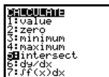
Figure 6e: Press the [2nd] [TRACE] buttons on your calculator and choose the "intersect" capability.
